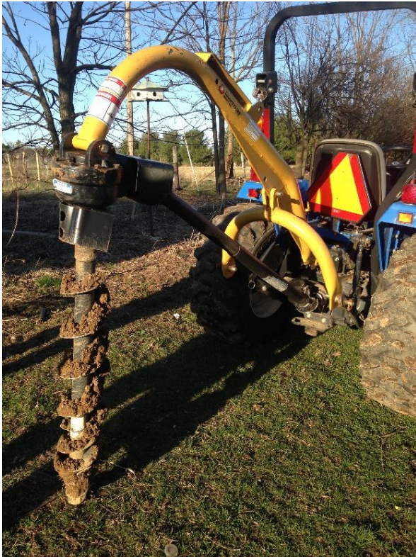
Post hole digger. Much faster than doing it by hand.
